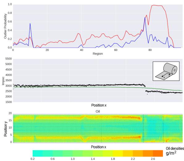
Fig. 3. Results for coil #1 Top: GLOSS (red line) and LoOP (blue line) outlier probabilities for each of 99 consecutive coil segments. Middle: IMPOC measurements over the whole length of the coil, both for this particular coil (black) and averaged over its 20 global neighbors (green). Bottom: Oil level measurements visualized in 2D, representing the entire surface of the coil.
